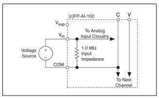
Figure 4. Voltage Source without External Power Supply
