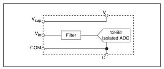
Figure 3. [c]FP-AI-102 Analog Input Circuit, One Channel
