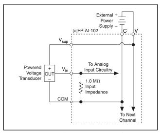
Figure 5. Voltage Source with External Power Supply
