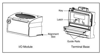
Figure 1. Installing the FP-AI-102
