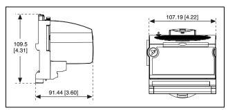
Figure 6. FP-AI-102 Mechanical Dimensions
